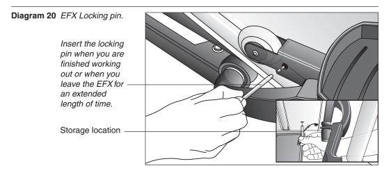
The locking pin secures the roller arm and keeps it from traveling up or down the ramp. Pull firmly on the pin to slide it out of the ramp. A lanyard is attached to the locking pin and ramp. Refer to Diagram 20.
